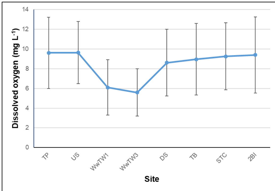
Figure 4.48 Annual dissolved oxygen concentrations, upstream and downstream of WwTW. WwTW2 excluded as composite collection vessel is refrigerated. Error bars represent \pm 2x St. Dev.
