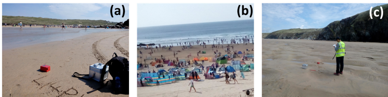
Figure 6. Field survey was conducted in the summer season: (a) shows typical distance between beach users and Tromino unit, (b) portable wind breakers deployed by beach users during the survey, and (c) member of staff using a high visibility jacket to indicate location and indicate beach users not to get too close to the unit while sampling (Source BGS).
