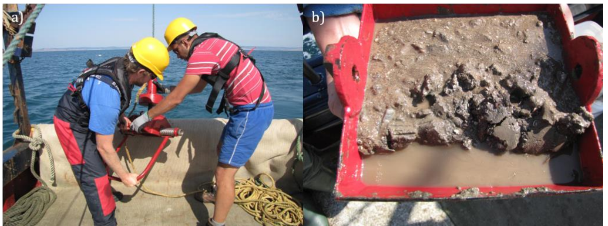
Figure 4.4: a) Shipek grab being prepared for deployment, and b) undisturbed unwashed seabed sample.
