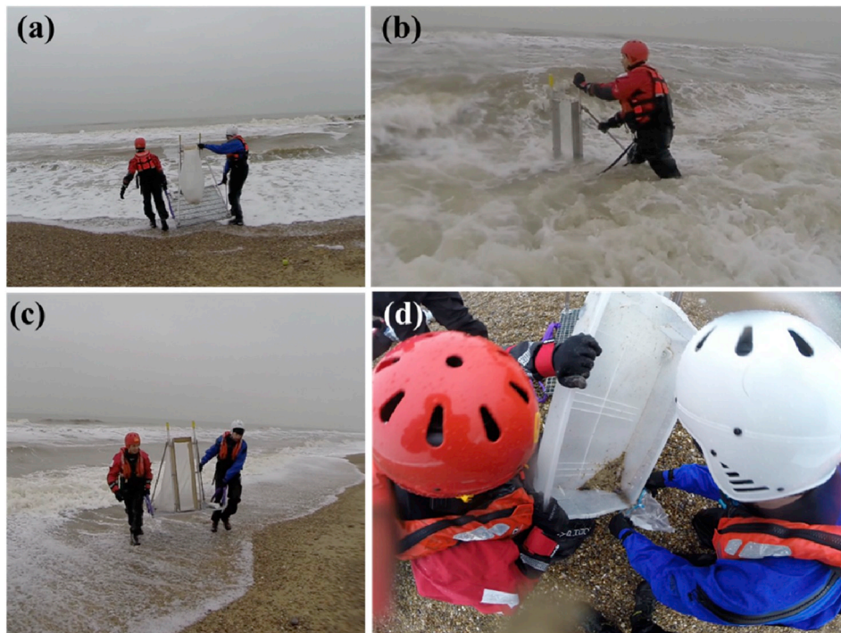
Fig. 2. Photograph showing traps in operation: (a) transportation from dry beach to sampling location; (b) during sampling one operator holds trap in place by standing on top of the reticulated base; (c) once sampling is finished, two people recover the trap and (d) transfer the collected sediment to a bucket first and a labelled plastic bag for storing and sediment size analysis.
