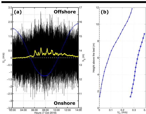
Figure 4. Cross-shore velocity ( $U_C$ ) and pressure measured by SIG1 during very oblique storm conditions ( $H_S = 4$  m and  $\Theta_p = 27^\circ$ ). (a) Instantaneous (black), 5-min time-averaged (yellow) depth-averaged  $U_C$  and 5-min time-averaged pressure (blue). (b) Vertical profile of instantaneous  $U_C$  time-averaged over low (circles) and high (crosses) tide.
