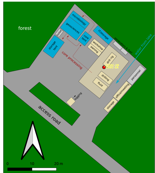
Figure 3. Sketch of the COSC-2 drill site. The area is approximately 1600 m 2 large, with the northwestern half used for the science operations (blue), parking, and storage and the southeastern half used for the technical operations (yellow) and common facilities. The route of the core from drilling deck to storage is marked in red.
