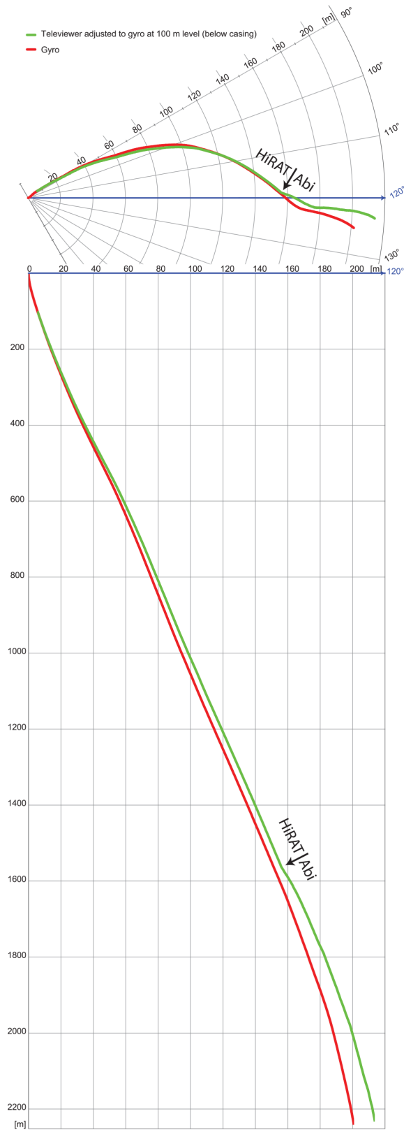
Figure 5. Borehole path of the COSC-2A borehole, based on surveys with a north-seeking gyro (red; REFLEX GYRO SPRINT-IQ™) and the orientation sensors of acoustic televiwers (green; derived from accelerometers and magnetometers). The televiwer data are spliced at 1570 m, with data from the Robertson Geologging High-Resolution Acoustic Televiwer (HiRAT) above this depth and from the ALT Abi43 televiwer below this depth.
