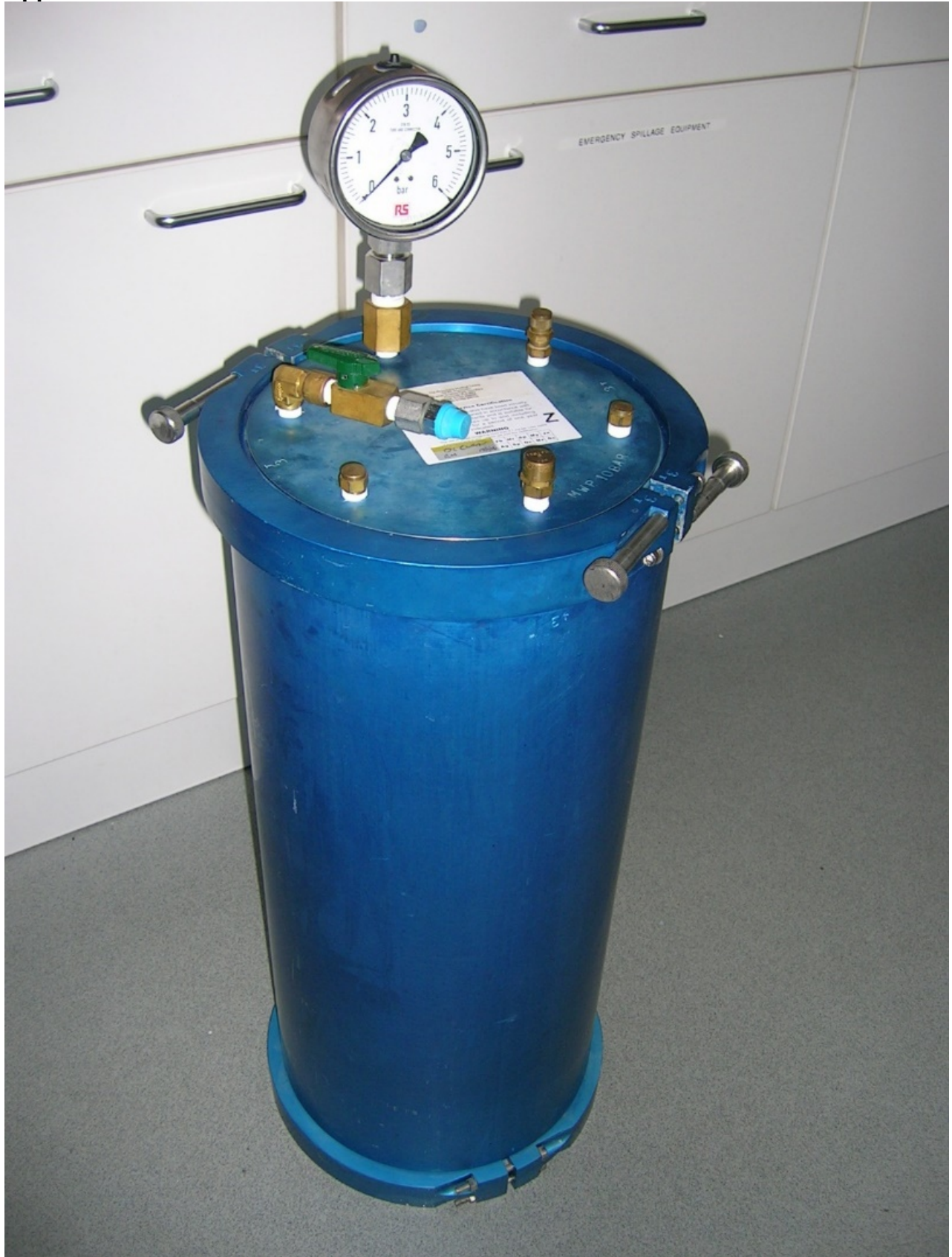
Figure S1 – Chamber used to culture bacteria under increased atmospheric pressure
