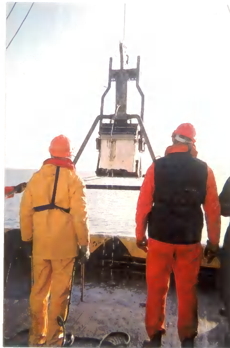
Figure 2.4 Photographs of (a) a Day grab after the collection of a surface sediment sample and (b) a box corer being recovered after the collection of a sediment sample.
