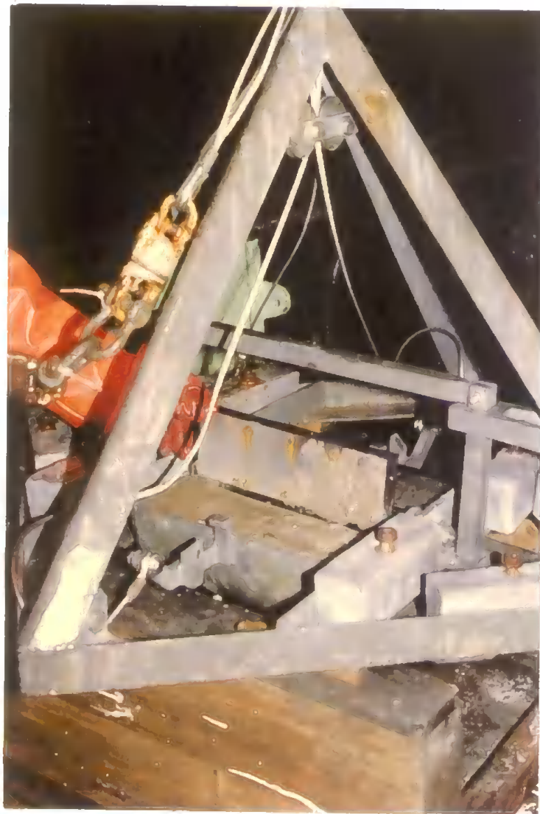
Figure 2.4 Photographs of (a) a Day grab after the collection of a surface sediment sample and (b) a box corer being recovered after the collection of a sediment sample.
