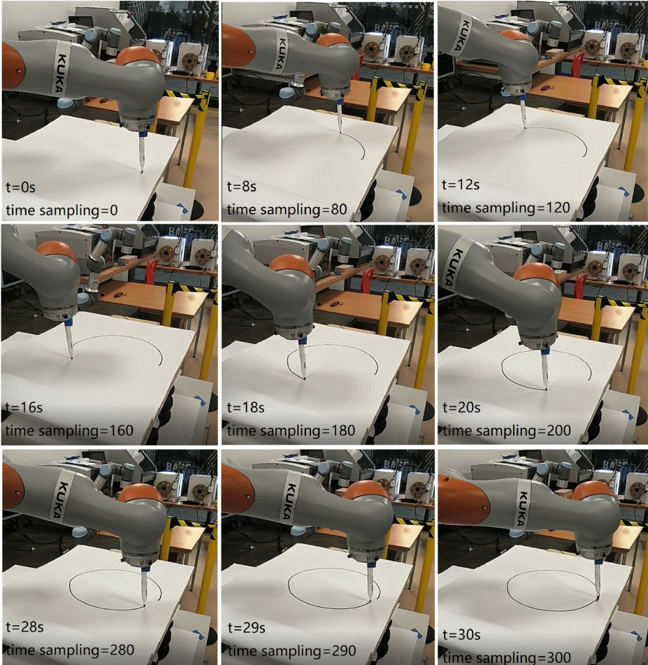
Figure 8. Snapshots from experiments of the KUKA iiwa robot while drawing a circle path with locked joints based on SFTMP.
