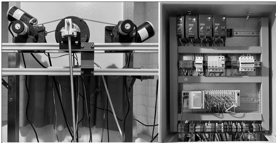
Fig. 2. Test rig and controller. Panel A: Tendon worm-drive link test rig on stand. Panel B: DIN rail Beckhoff EtherCAT panel.
