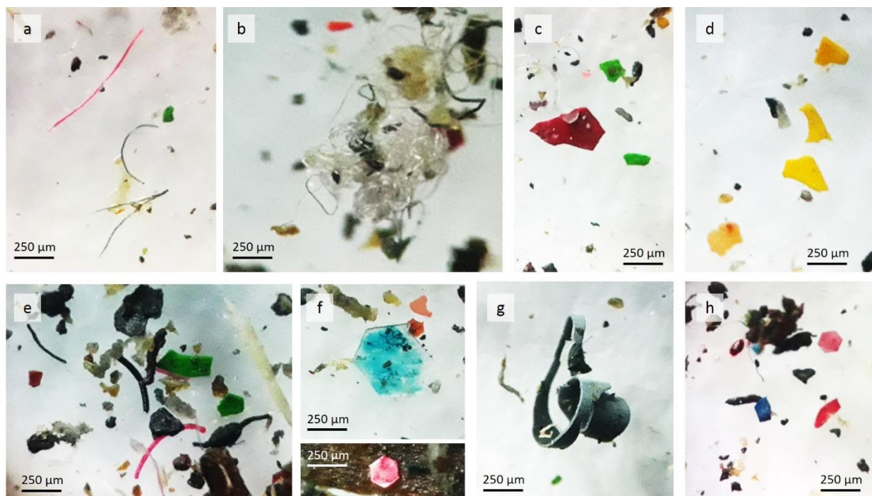
164 Figure 2. Optical microscope images of different types of microplastic retrieved from dust 165 samples collected in various schools. Plastic fragments of varying colours and sizes are evident 166 in all images, synthetic fibres are evident in (a), (b), (c), (e) and (f), black rubber fragments are 167 evident in (e) and (h), and hexagonally-shaped primary plastics are evident in (f) and (h).
