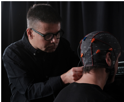
FIG. 1. Brain activity can be read using electrodes strategically placed on the human scalp.
