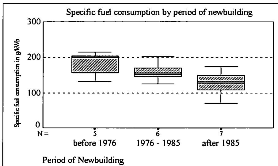
Figure 2-18 Specific fuel consumption of ferries by period of newbuilding
