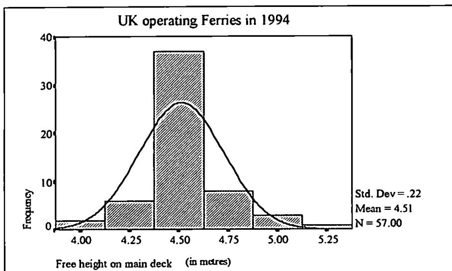
Figure 2-12 Free height on main deck available on UK ferries
