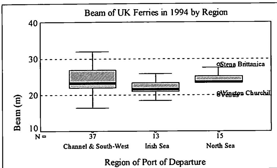
Figure 2-11 Beam of UK ferries by region
