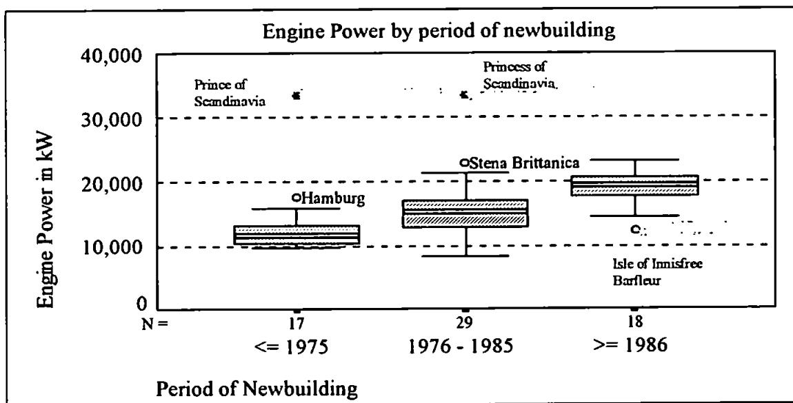
Figure 2-19 Engine power by period of newbuilding
