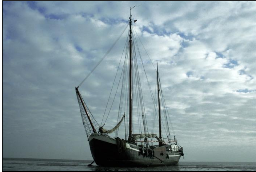
Plate 3.14 'De Walvisch (1896) Dutch Klipper with Dutch monument status' Note the lee boards. Courtesy of Zatorski A
