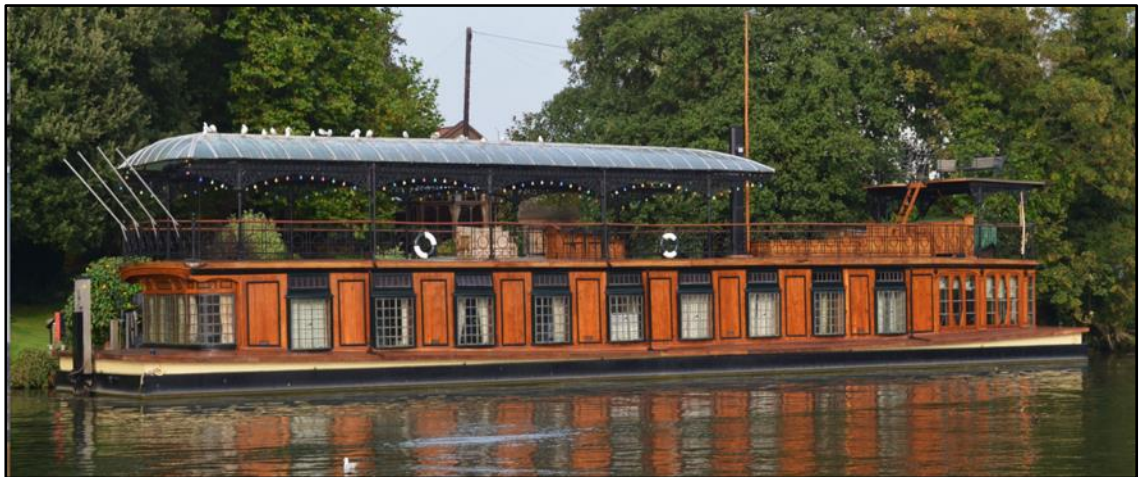
Plate A 'Astoria', (1911) Houseboat, Hampton; early houseboat type purpose built primarily for summer use. This type of vessel would have been towed by steam, tug, horse, or mule on the non-tidal Thames. (2018) Courtesy of photographer J. Beard.
