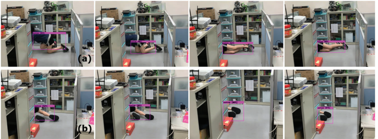
Figure 15: Fall process chart of body occlusions. (a) 50% and (b) 70% occlusions.
