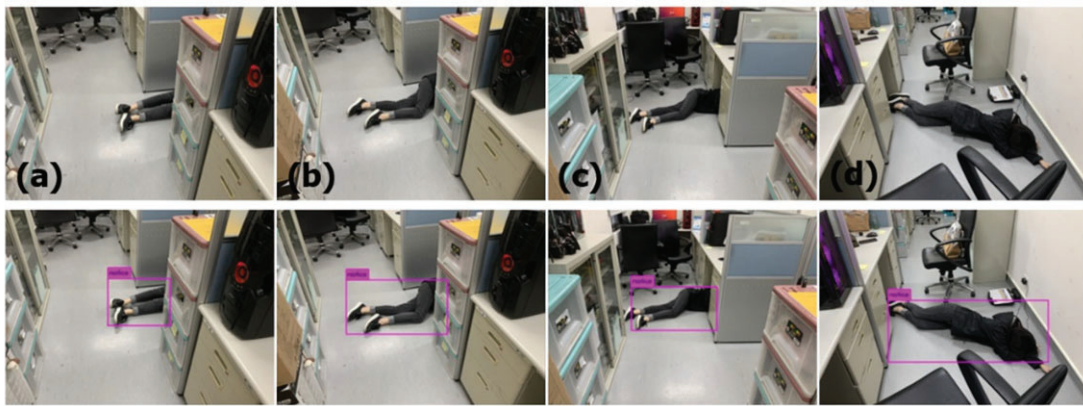
Figure 10: Anomaly detection with various occlusions. (a) 70%, (b) 50%, (c) 30%, and (d) 0%.
