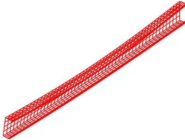
Figure 4.2 Lateral-torsional buckling mode of a 3-meter-long CFS beam (without holes) in CUFSM. ( h=200 mm, b=70 mm, c=20 mm, t=2 mm)
