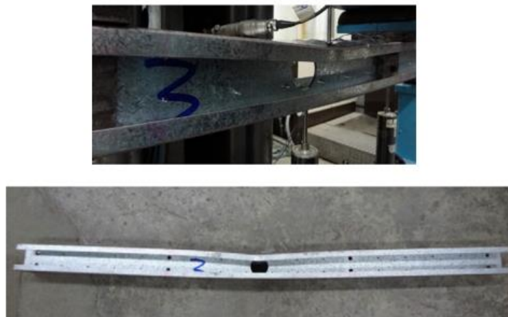
Figure 2.13 Ultimate stage of distortional and flexural buckling of CFS built-up beams with web perforation in the four-point bending tests. (Wang and Young, 2015c)
