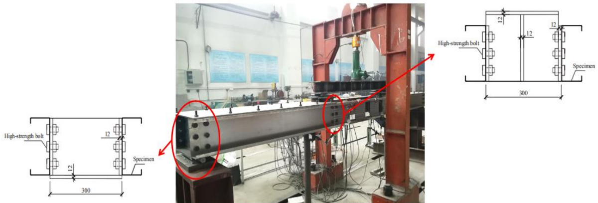
Figure 2.8 Four-point bending test rig (Zhao et al., 2019)
