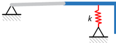
Figure 2.2 Distortional buckling model proposed in EN-1993-1-3 (2006)
