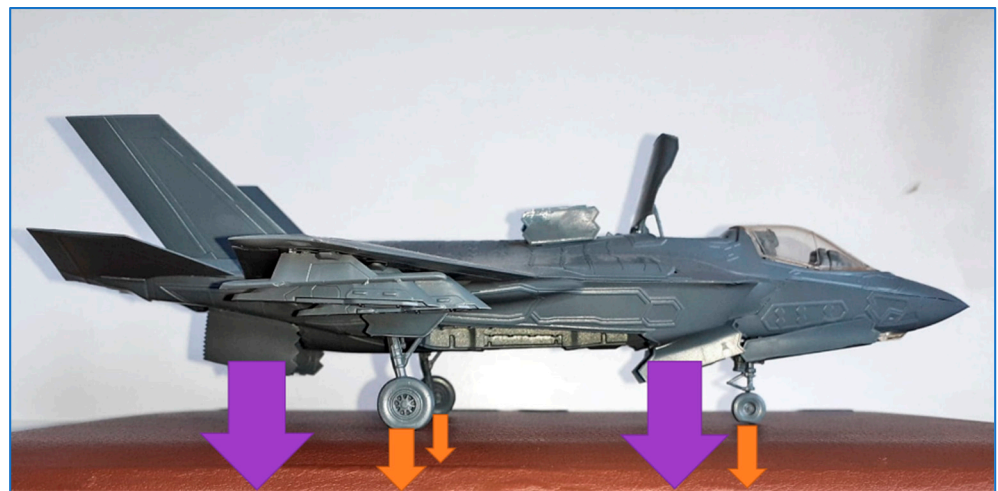
Figure 5. Locations of the pressures applied to the deck during a vertical landing.
