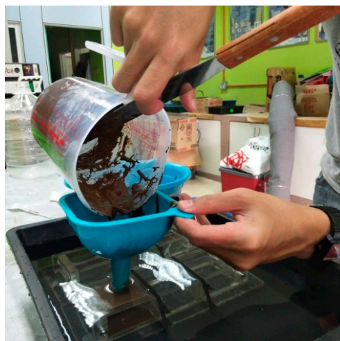
Figure 1. AAFA paste poured into mould in seawater.
