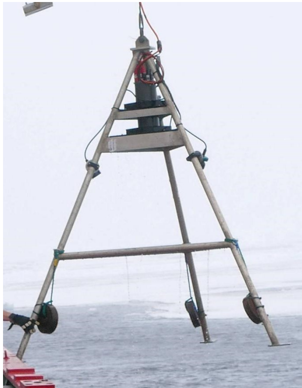
Figure A.1: British Antarctic Survey's Shallow Underwater Camera System (SUCS).
