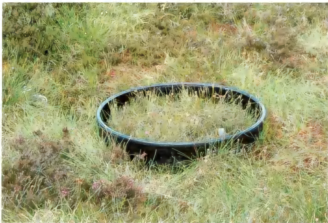
Plate 4.6: Examples of the lysimeters installed by Dundee University at Dun Moss. The lysimeter is the green circular object; within this is a dipwell (grey pipe). To the left of each lysimeter is an anchor to measure peat movement. Diameter of each lysimeter ca. 60 cm. For details of vegetation, see Table 4.3.
