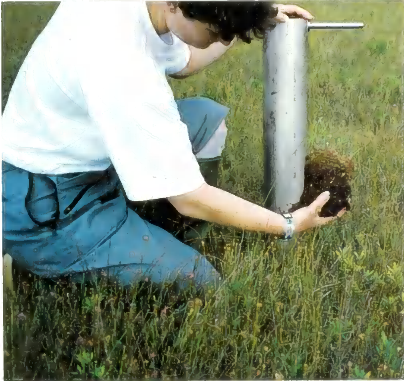
c) The core is carefully removed and placed on a clean cutting surface
