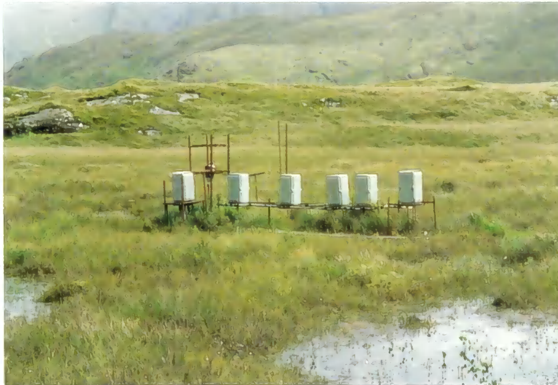
Plate 4.5: Water table recorders installed by SNH across a hummock-hollow complex, Coladoir Bog. The comparable complex is out of the picture, on the right hand side, on a line with the depth recorders.
