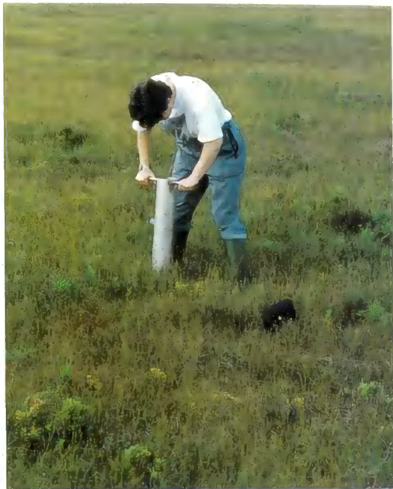
a) The steel cylinder is driven through the Sphagnum into the peat layer.
