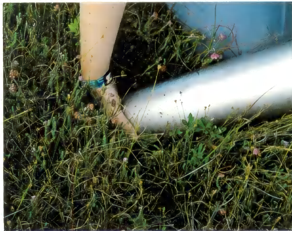
b) The core is retrieved and supported within the cylinder.
