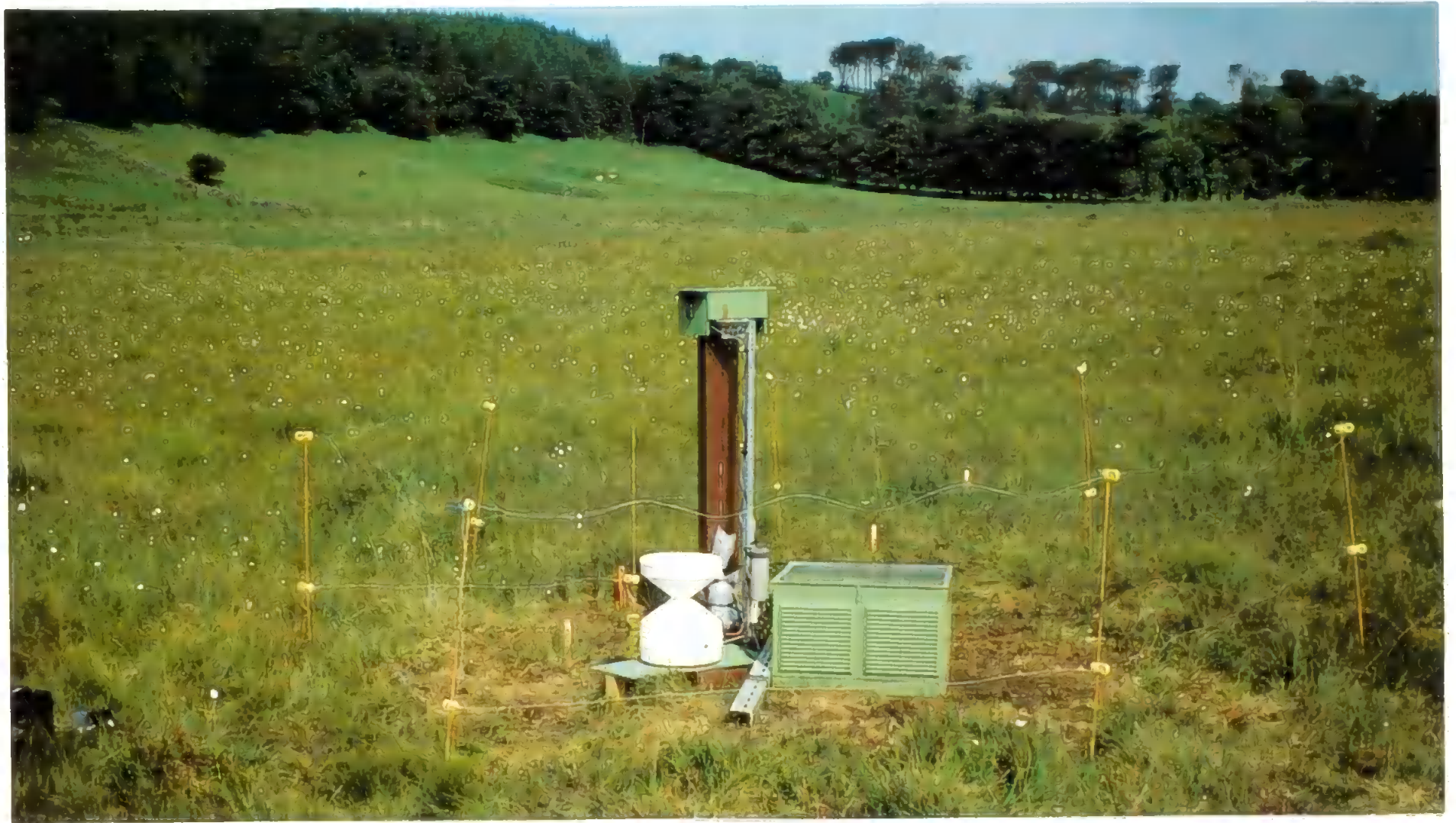
Plate 4.3: The automatic recording station at Tor Royal. The white funnel is the rain gauge; the conductivity and temperature probes and batteries are contained in the green box. The potentiometer and float for recording water table movements are housed in the brown pipe. An electric fence surrounds the equipment.
