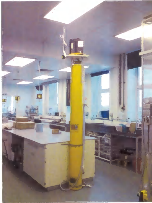
Figure 2.10 - Automated settling tube used to determine the sediment fall velocity distribution.
