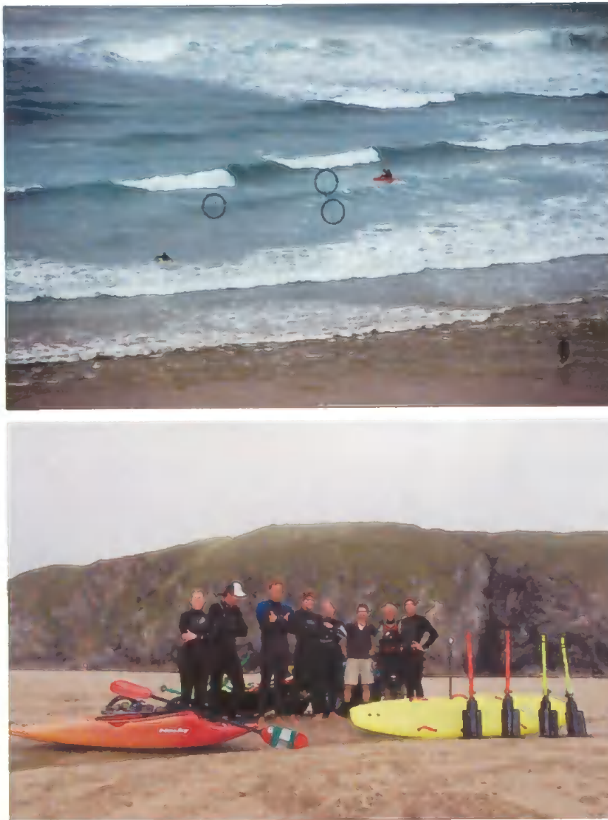
Figure 6.5 – Photograph (above) of GPS drifters in the surf zone during the experiment. Drifters circled in black, with waterline at the base of the mast. Photograph (below) manpower required to safely conduct the experiment without PWC assisted pick-up.
