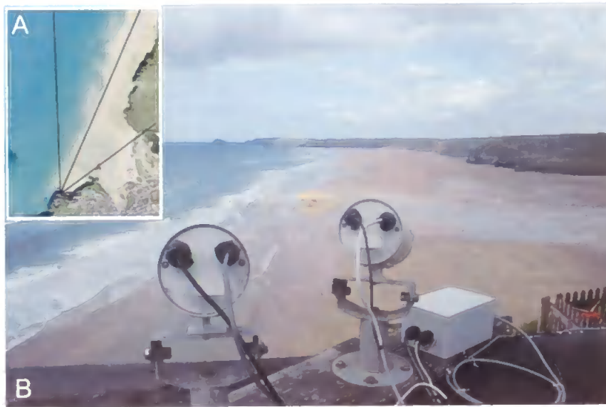
Figure 2.6 - Argus video cameras at Perranporth at an elevation of 47.87 mODN (B) and indication of the extent of the field of view (inset A).
