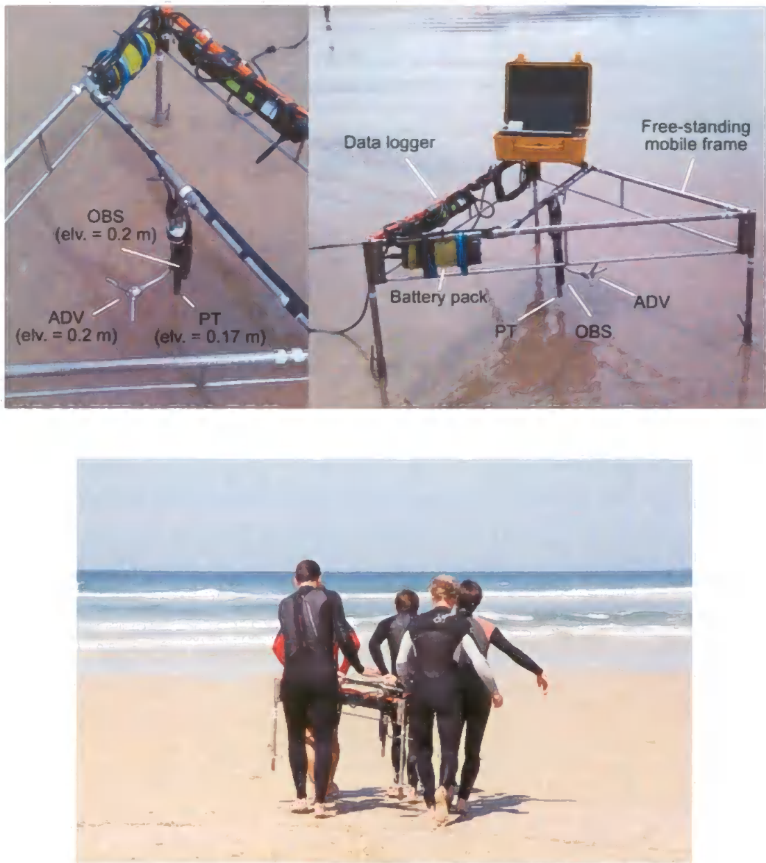
Figure 6.3 – Free-standing mobile instrument frame (one of two) showing Nortek Vector 3D – Acoustic Doppler Velocimeter (ADV), Pressure Transducer (PT) and Optical Back Scatter probe (OBS). Image on left indicates sensor elevations above the bed. Bottom image shows instrument frame deployment.
