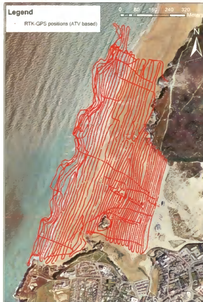
Figure 2.4 - Image showing typical survey track at Perranporth beach. Alongshore orientated lines enable maximum morphological coverage throughout the low-tide region due to rapid cross-shore tidal translation rates.
