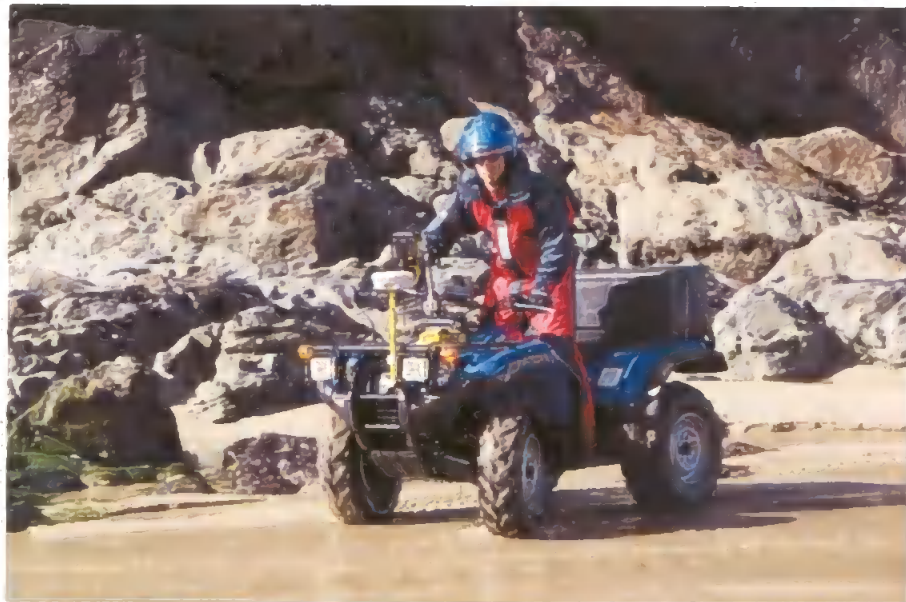
Figure 2.2 - ATV mounted RTK GPS system in use conducting a beach survey. Trimble 5800 dual frequency receiver is mounted on front bars and TSC survey controller on the handlebar mount. All data links are wireless via Bluetooth.
