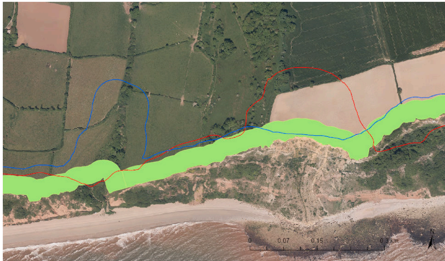
Fig. 5. Variations between erosion mapping. Blue line indicates SMP 2105 indicative erosion extent, green banding indicates NCERM 5th %ile 50–100 year erosion banding and red line shows Plymouth University/East Devon DC collaboration 100 year erosion extent using cliff face volume analysis and UKCP18 SLR/Acceleration in SLR projections. (For interpretation of the references to colour in this figure legend, the reader is referred to the Web version of this article.)
