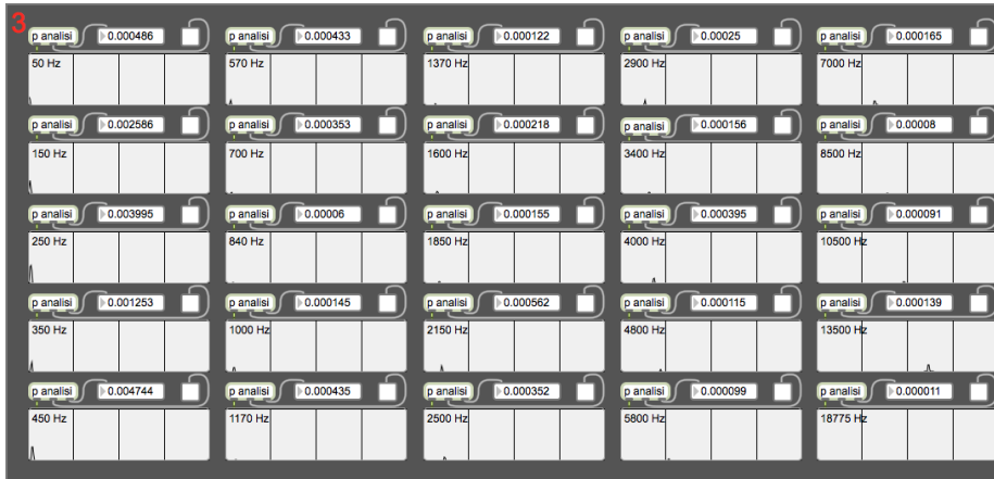
Fig. 13 Area 4, screen 25 resonators with their display, set each on the centre frequency of the critical band corresponding second Eberhard Zwicker mode
