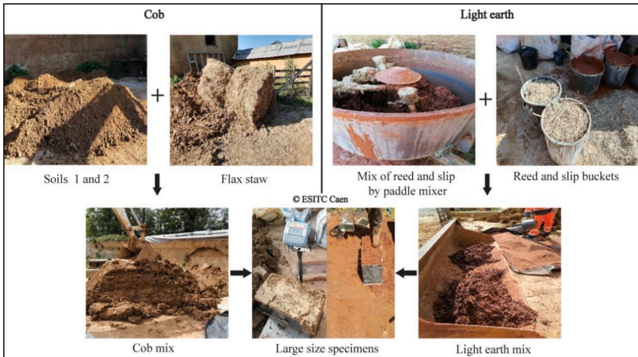
Fig. 4. In-situ preparation of cob and light earth.
