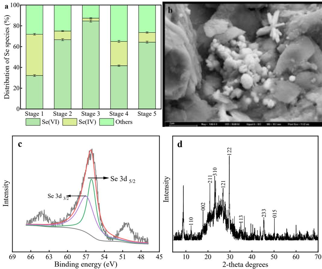
**Fig. 2.** Characterization of products from Se(VI) bioreduction. (a) Selenium speciation percentages in the effluent. (b) SEM, (c) XPS, and (d) XRD analysis of the precipitates after reaction. SEM: Scanning electron microscope; XPS: X-ray photoelectron spectroscopy; XRD: X-ray diffraction.
