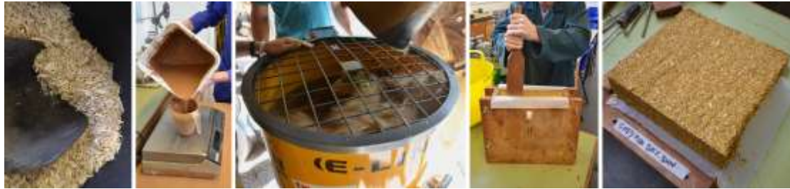
Figure 1. Sample preparation stages. (left to right. Cut fibre, weighed slip, mechanical mixing, hand tamping, completed sample)
