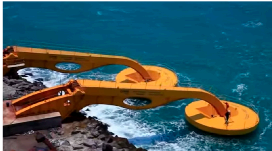
Figure 5. WAB-type WEC operating in Pecem. Image taken from Ref. [32] “Cascajo, R.; García, E.; Quiles, E.; Correcher, A.; Morant, F. Integration of Marine Wave Energy Converters into Seaports: A Case Study in the Port of Valencia. Energies 2019, 12, 787.” Copyright 2019 Author(s), licensed under a Creative Commons Attribution (CC BY 4.0) license.
