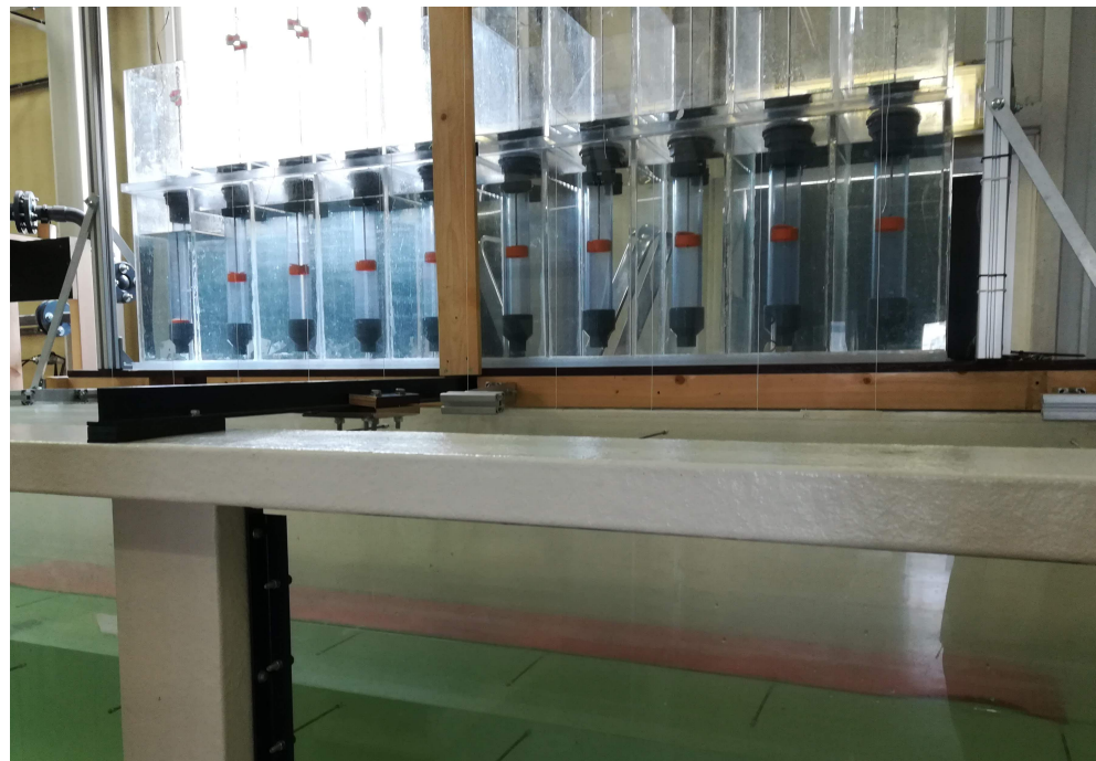
Figure 19. Laboratory demonstration of the flexible floater (red silicone sheet inside the tank) connected to the MP 2 PTO system at the University of Groningen.
