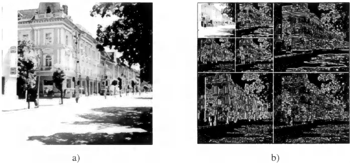
Fig. 3.8. A 2-level wavelet decomposition using the 2D version of Mallat's algorithm. a) The original image b) The 2 levels of detail coefficients and the smoothed data.
