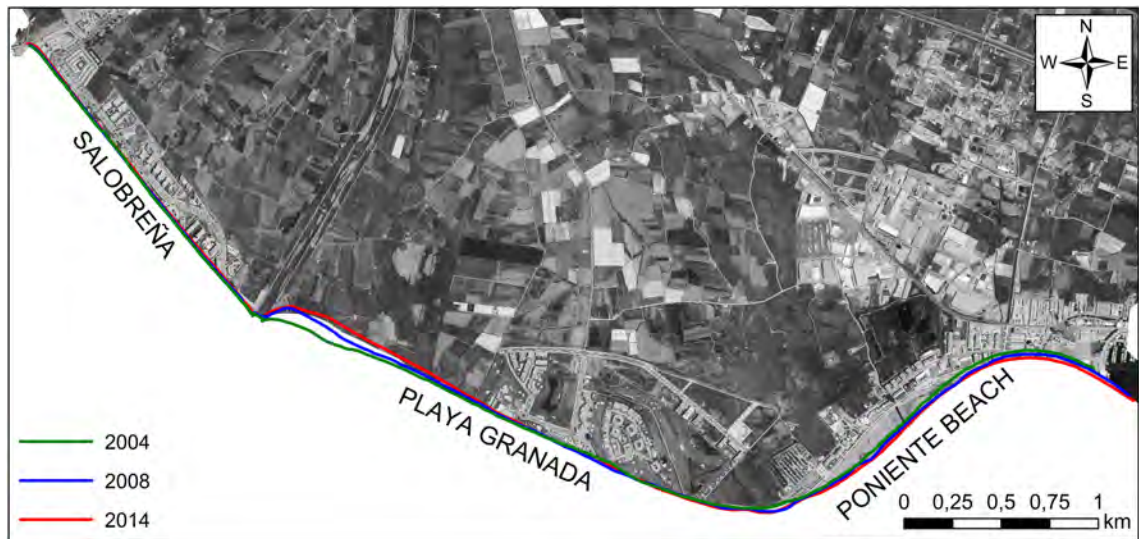
Fig. 4.10 Shoreline evolution since the Guadalfeo River damming in 2004. Rodriguez-Delgado et al. (2018b).
