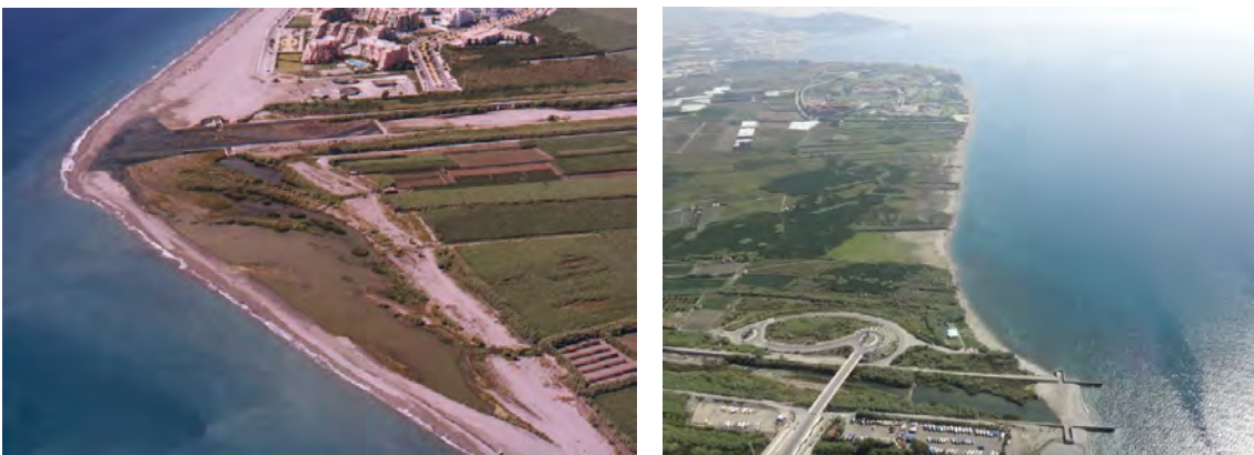
Fig. 4.8 Aerial photographs of the Guadalfeo River Delta before (left) and after (right) river damming. Rodriguez-Delgado et al. (2018a).
