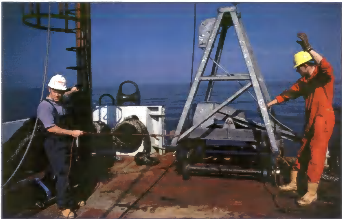
Figure 7a. Deployment of a 0.2 m 2 Hamon grab.
