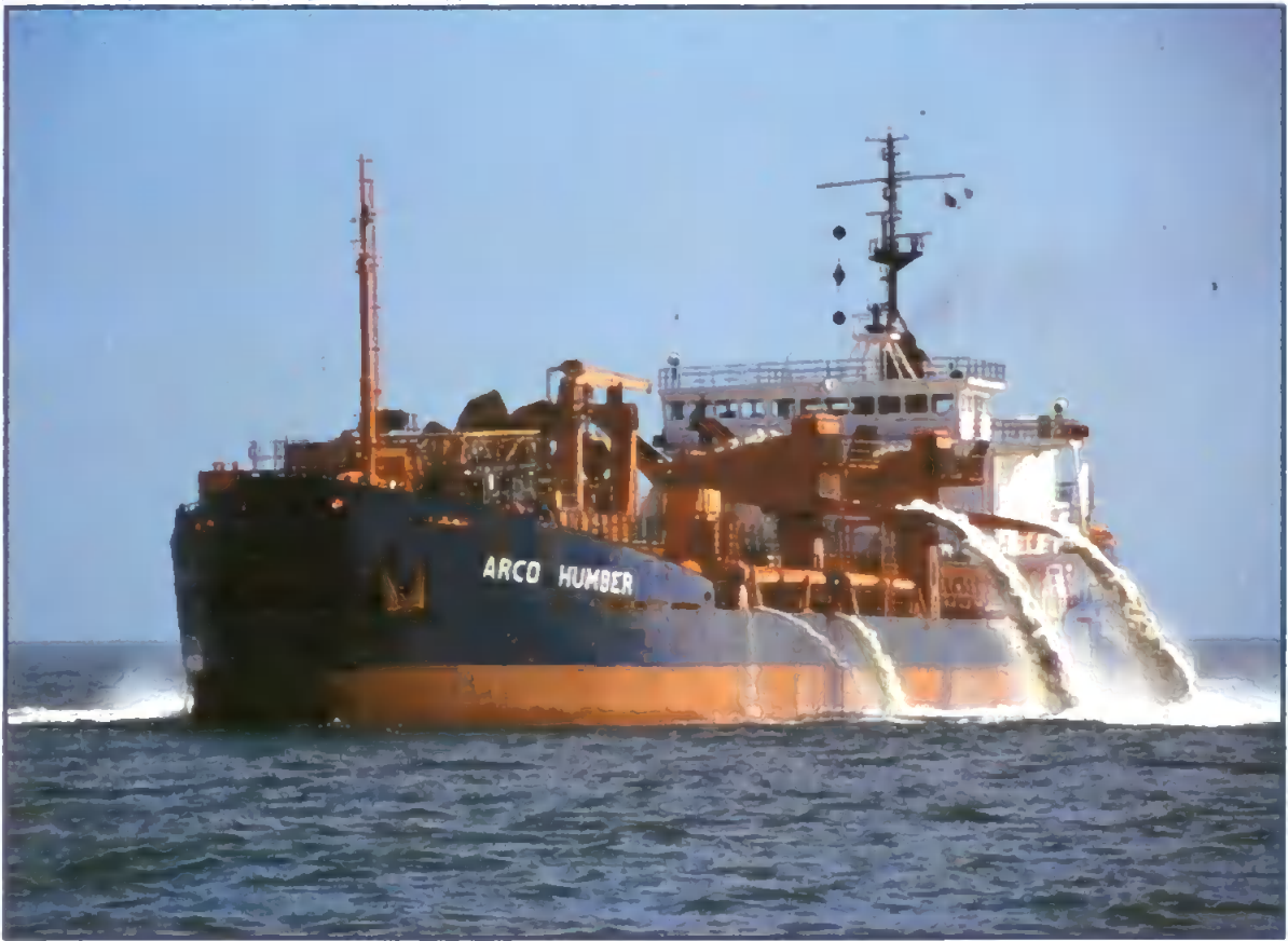
Figure 69. Trailer dredger (Arco Humber) operating in the North Sea, showing material rejected overboard after screening.
