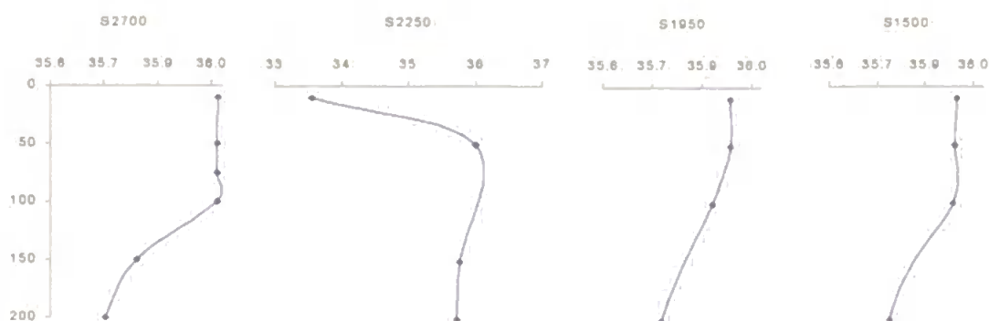
Figure 103. Vertical profiles of salinity in the upper 200m of M43/2 slope and offshore stations S1500, S1950, S2250 and S2700. Note: y-axis is depth (m).
