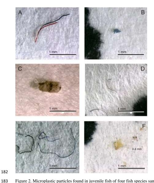
Figure 2. Microplastic particles found in juvenile fish of four fish species sampled from four mangroves in KwaZulu-Natal, South Africa. A: particles of rayon (red and blue), B: blue fragment of PVC, C: opaque fragment of PVC from Durban Harbour mullet, D: polyester fibre, E: rayon fibres and F: polyethylene fragment from a thornfish in Umgeni.
