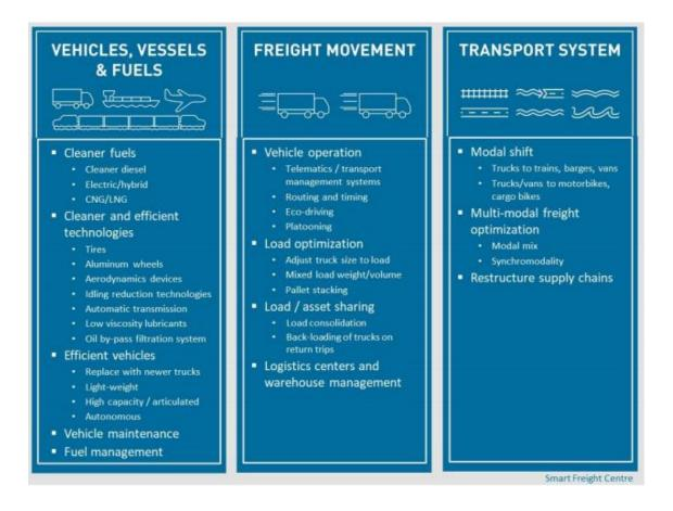
Figure 8-2 Technologies and measures relevant to road freight carriers Source: SFC (2016), p.7
