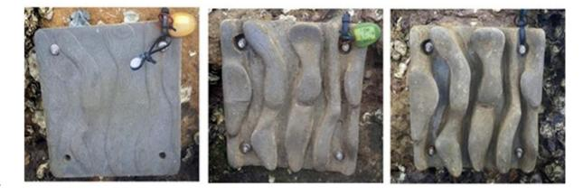
Fig 2: The three experimental treatments: a) flat, b) 2.5 cm complex, c) 5 cm complex.
