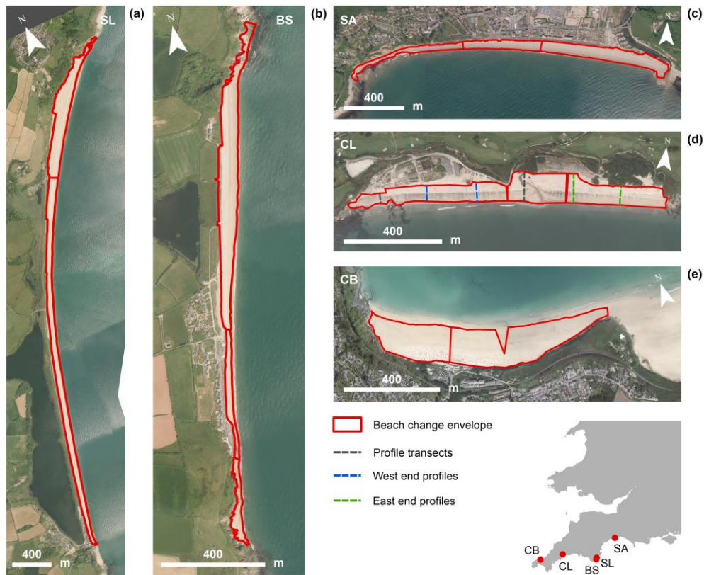
Figure 2. Beach Change Envelope (BCE) used for alongshore budget segmentation estimations shown for: Slapton Sands (a); Beesands (b); Seaton (c); Carlyon Bay (d); and Carbis Bay (e). The profiles used for calculating beach volumes representative of the two beach extremities for Carlyon Bay are also indicated.
