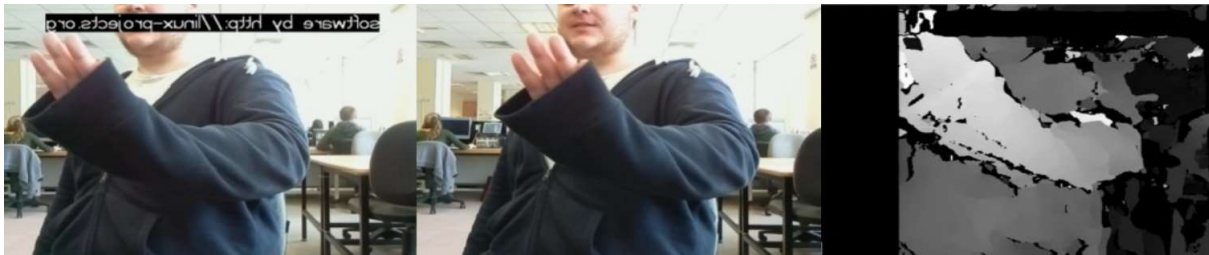
FIGURE 4 Stereo images and resulting disparity map.
