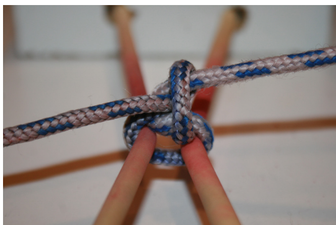
Figure 12 Initial effect of pulling on one end of reef knot causing initial loosening.
