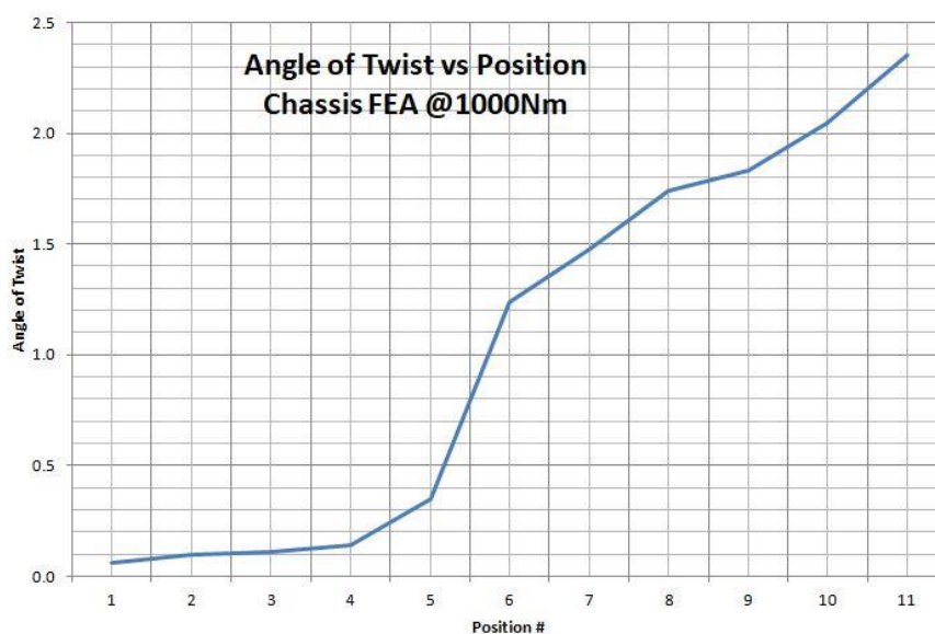
Graph 3: Chassis FEA: sensor position against twist angle
