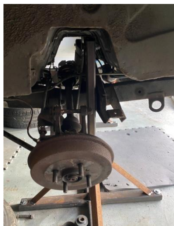
Figure 19: LH rear fixture bolted to the floor and chassis damper mount
