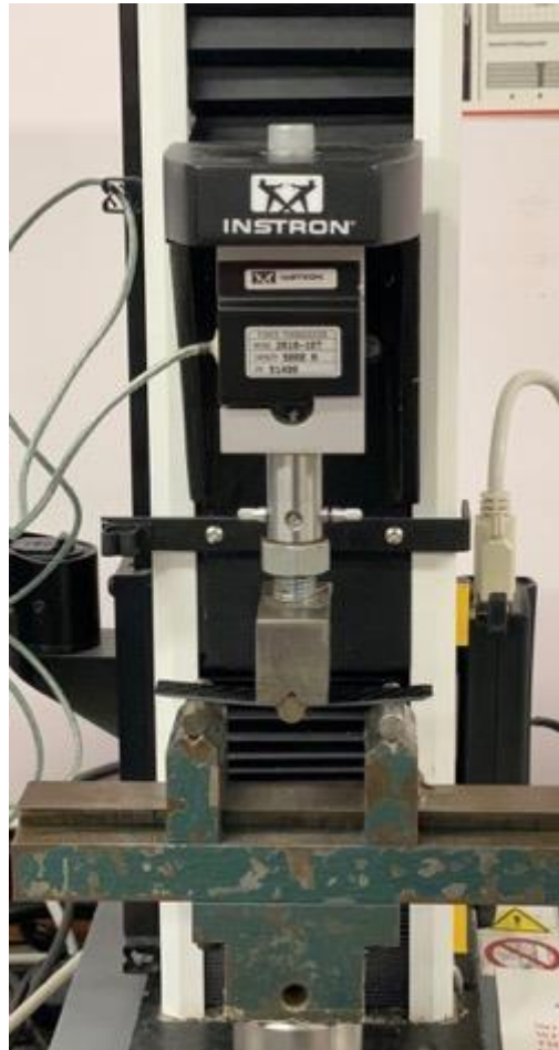
Figure 35: Instron testing machine, performing 3 point FLEX test for the individual coupons which were cut from the composite plate.
