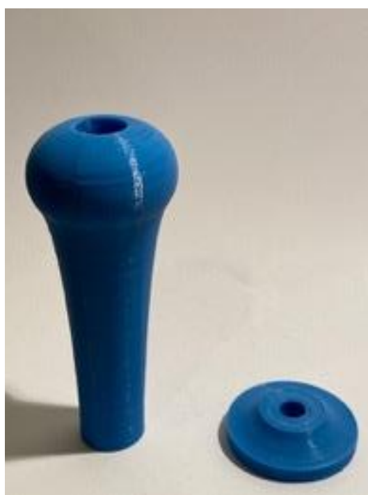
Figure 30: Shows the first prototype of the Hand Grip and Large Washer after being 3D printed from PLA. These two components will be held together by a titanium bolt and then integrated into the composite blade.
