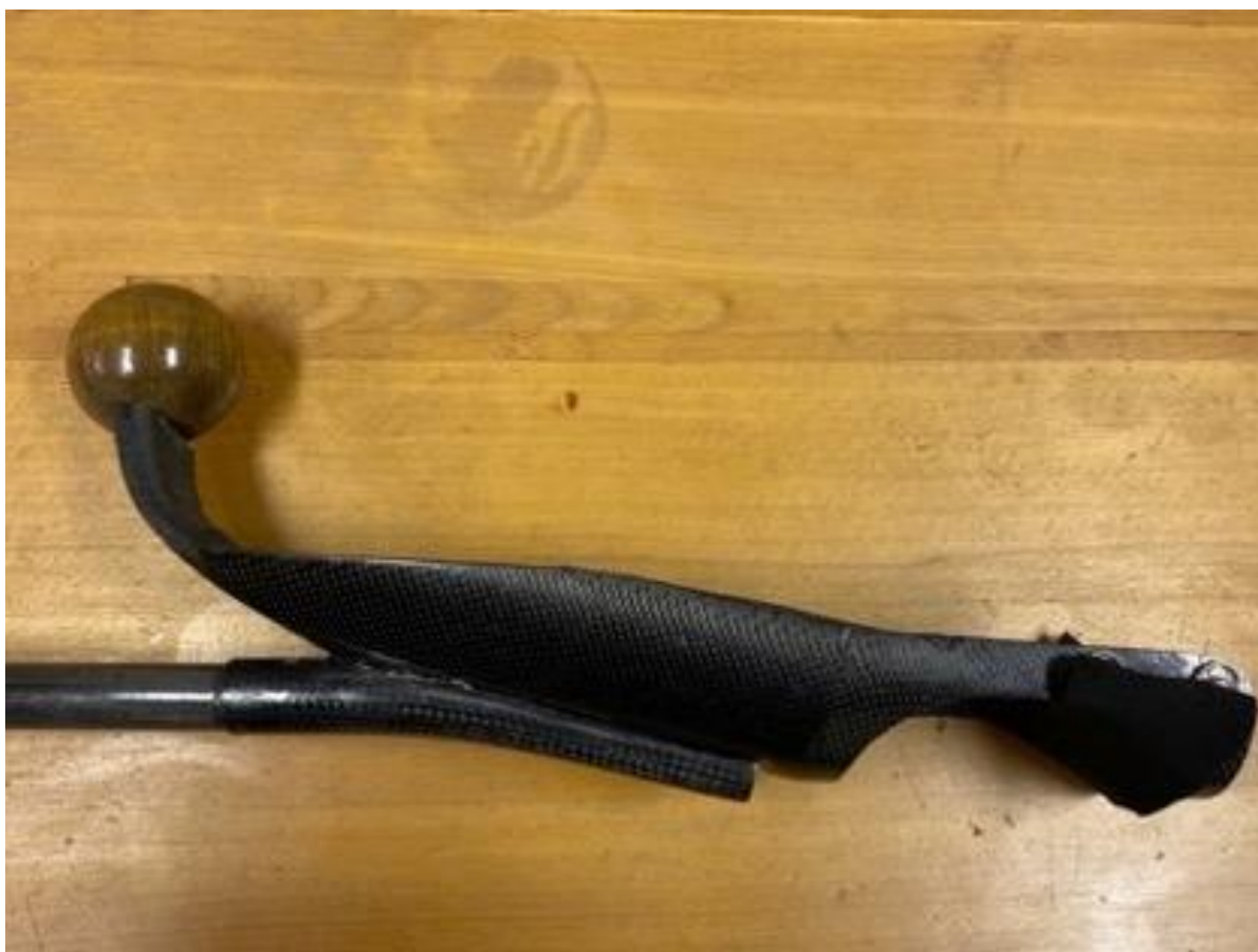
Figure 2: The overall measurements of the crutch were not exact to the athlete's specification, meaning it was too tall, causing the crutch arm support to press into the athletes under arm, making it uncomfortable for use, these forces can also cause long term damage like crutch palsy which for anyone who uses crutches every day is not acceptable.
