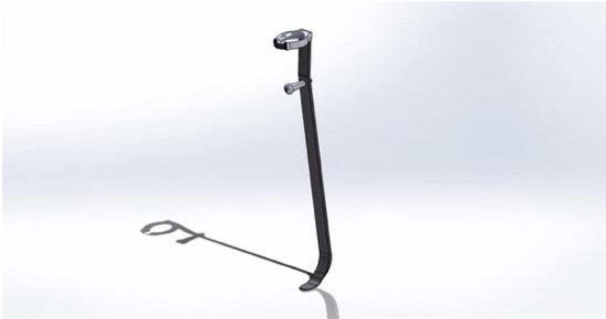
Figure 31: The final crutch assembly, consisting of the carbon fibre blade with sub-assemblies for the Hand grip and Arm Support (cuff). This model was produced to show the athlete and sponsors what the final crutch would look like allowing feedback before production. Unfortunately, due to Covid-19 the athlete has been unable to try the prototypes but will do so when possible before the final components are produced.
