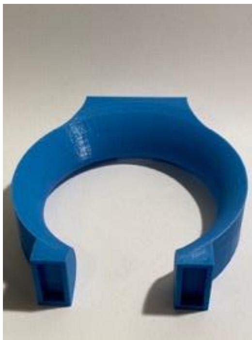
Figure 28: These prototypes were manufactured using PLA due to its low cost and easy access but most importantly no mechanical properties were required meaning the part could be printed with minimal fill to reduce cost and print time.
