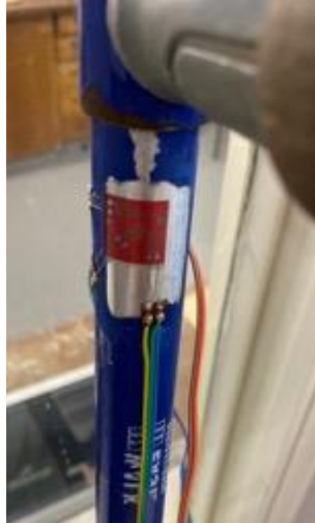
Figure 12: The attachment of the strain gauge to the current crutch. The process in which the strain gauge was attached involved cleaning the crutch by removing all rust and paint so the gauge could be attached directly to the aluminium tube.
