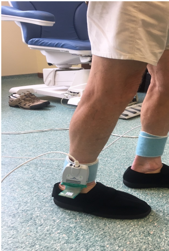
Figure 4.4 Participant using the Fscan system, insole and Pulman-house shoe
