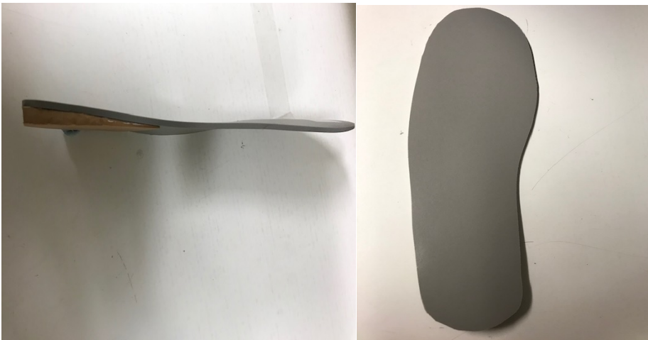
Figure 4.3 Active control insole from medial view and dorsal view
