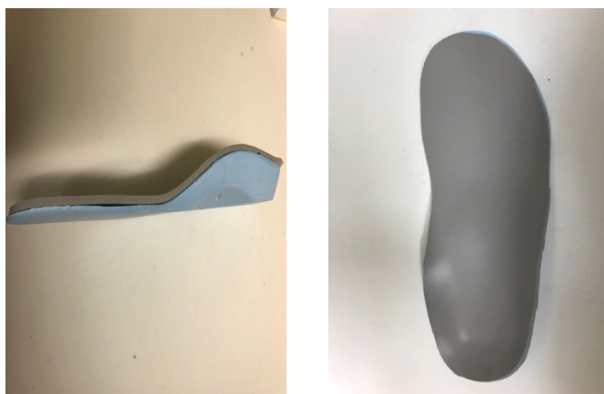
Figure 4.2 Optimised insoles from medial view and dorsal view
