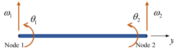
Fig.5 Beam element in local coordinate system
