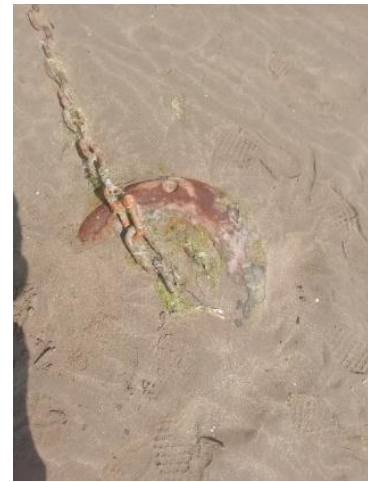
Plate 5. 10 Cement filled tyre connected to buoy, July 2019
