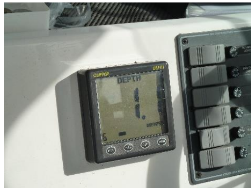
Plate 5. 4 Depth Sounder, located in the control room of Appledore – Instow Ferry, to the left of the steering wheel, October 2019
