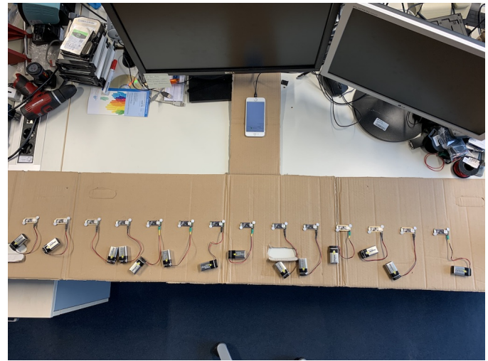
Fig. 3. Test setup for the main-test: In order to always have the same test conditions, the devices were positioned on a template (light brown). The smartphone can be seen in the top part of the figure in front of the monitor. In the bottom part the 14 battery powered Bluetooth sensor nodes are equally positioned in a row. To avoid slipping between the tests, the nodes were attached to the template. Each space between two nodes was approximately 6 cm and the smartphone was located about 29 cm from the nearest node. The space between the smartphone and the nodes was kept free.
