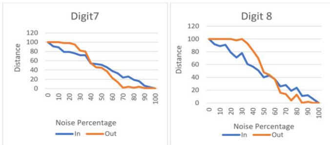
Figure 2. The blue line shows the calculated distances between input and noised input after adding noise. Orange lines show the distances between active columns encoded by SP for the reference input (without noise) and the output columns encoded by SP for a given noised input vector.
