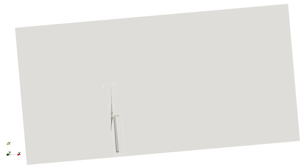
Figure 7: The entire domain has been rotated by 5^\circ , reflective of the shaft tilt, in order to produce a single-axis rotation about the rotor’s centre of rotation. All boundary and initial conditions are adjusted accordingly to maintain flow parallel to the ground.
