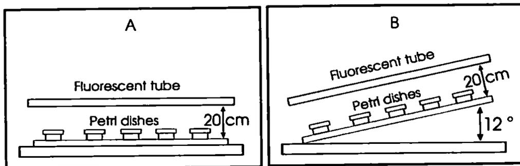
Figure 9.1: Schematic diagram of equipment to test geotaxis.
