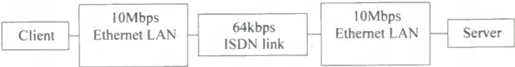
Figure 5.8 – Block diagram of the bottleneck bandwidth testbed
