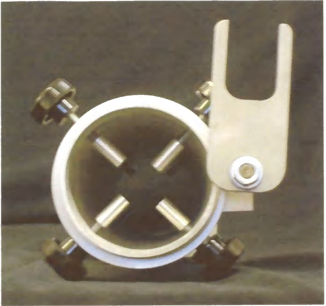
Plate 2.4: Plan view of the axial alignment frame
