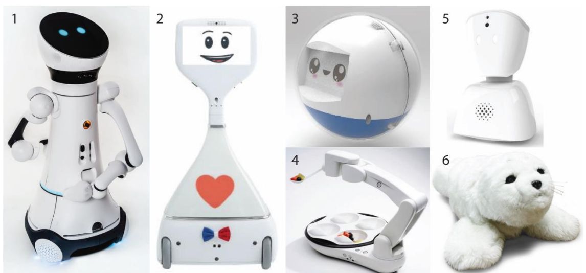
Figure 7; Assistive robots available in the market. 1 Care-O-bot; domestic robot assistant, 2 Cuttii; telepresence robot for older people, 3 Leka; a therapeutic robot for children with developmental disorders, 4 Obi; robotic feeding device, 5 AV1; robotic avatar for children with long term conditions.
