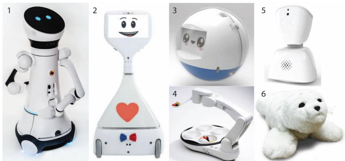
Figure 1. Assistive robots available in the market. 1 Care-O-bot; domestic robot assistant, 2 Cutii; telepresence robot for older people, 3 Leka; a therapeutic robot for children with developmental disorders, 4 Obi; robotic feeding device, 5 AV1; robotic avatar for users with long-term conditions, 6 Paro; therapeutic robot.
