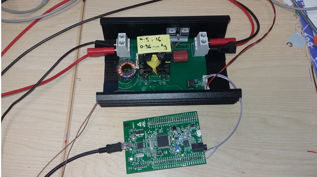
Fig. 4.6: Constant output voltage final prototype assembly with STM-Discovery switching control board
